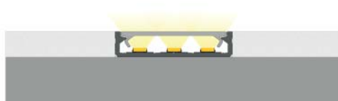
The end result of the installation of SOLIS profile with WIDE cover groove mounted between the boards
