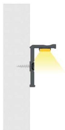
The end result of the installation of profile E using a mounting screw
