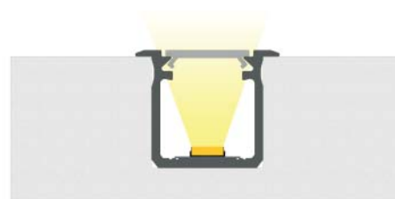
The end result of installation of groove mounted profile G with a BASIC cover
