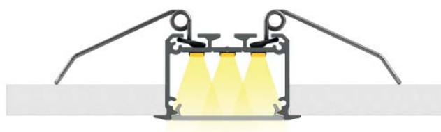
The end result of the installation of INSO profile with WIDE cover groove mounted between the boards
