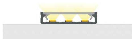
The end result of the installation of SOLIS profile with WIDE cover using double-sided tape
