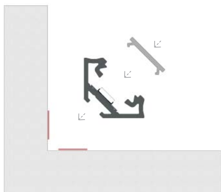
Installation instructions for angular profile C with a BASIC cover using double-sided tape
