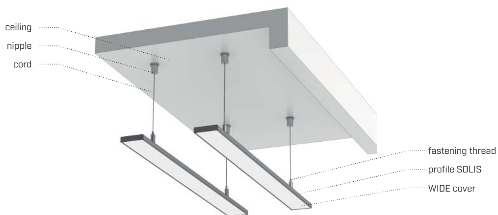
Installation of SOLIS profile as a pendant lamp
