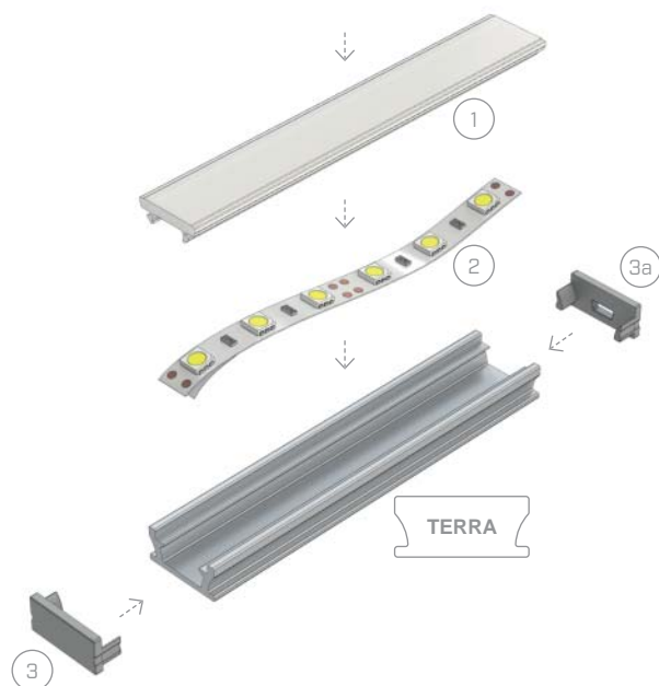
Assembly scheme for the elements of the lighting system using TERRA profile and (1) a floor cover, (2) LED strip, (3) end cap without hole (3a) end cap with hole
