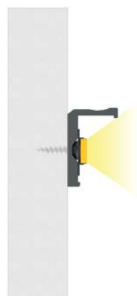
The end result of the installation of profile F using a mounting screw
