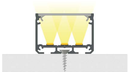
The end result of the installation of iLEDO profile with WIDE cover using mounting screw
